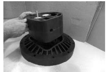
Step 3 Install flanges into the air chambers
