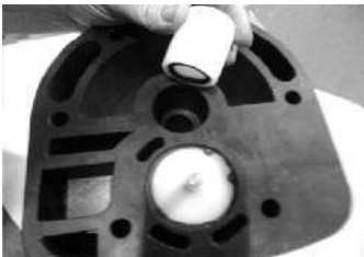
Step 1 Install bearings inside the central block reception
