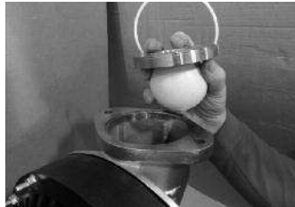
Step 5 Install ball valves, ball seats, o-rings
