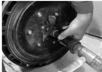
Step 4 We push outwards the air valve so that it exits the central block
