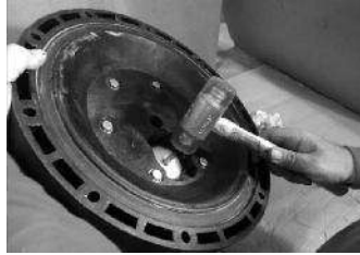
Step 2 From the one side we push the air valve shaft
