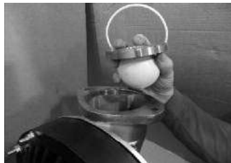
Step 2 Remove the balls and the seats. Reverse the pump and remove the suction manifold with the same way
