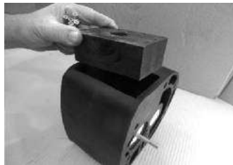
Step 2 Install and screw the air exhaust cover onto the central block
