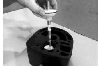
Step 3a From the opposite side we remove both cap and air valve shaft
